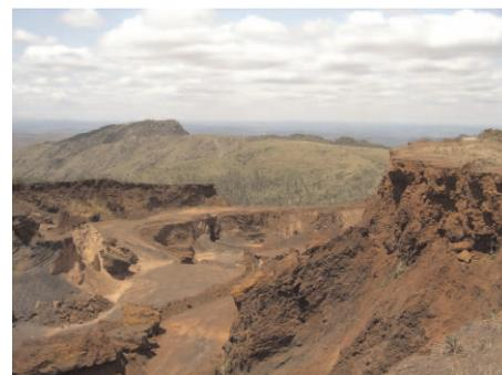
Partial view of an opencast iron-ore mine, showing the superficial crust removal.
